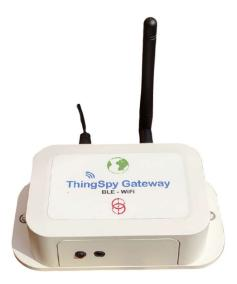
Thingspy Gateway is an IoT gateway device which uses various wireless protocol to monitor and track the assets in real-time. Thingspy gateway integrates a Bluetooth LE, Wi-Fi and an optional GNSS module which is ideally suited for different range of IoT applications. Another variant with LTE cellular
